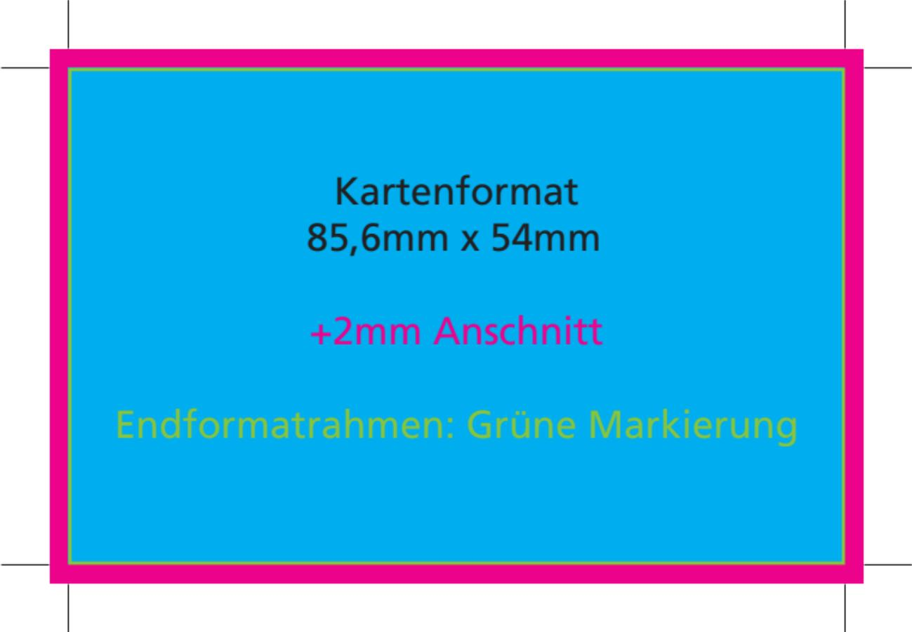
The diagram shows a central blue rectangle representing the card format. It is surrounded by a thick pink border. A thin green line is drawn inside the pink border, offset from the blue rectangle. The text 'Kartenformat 85,6mm x 54mm' is centered within the blue area. Below it, '+2mm Anschnitt' is written in pink. At the bottom, 'Endformatrahmen: Grüne Markierung' is written in green. The entire diagram is enclosed in a thin black frame with corner crop marks.
